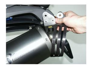
7. **For R 1200 GS & HP2 model:** tighten the carbon-fiber clamp onto the stock chassis hanging bracket on the frame - use the bolt and washers supplied in the Akrapovic kit. Do not fully tighten. Make sure the additional parts from the Akrapovic kit are correctly installed. **(Figure 11, 11a).**
